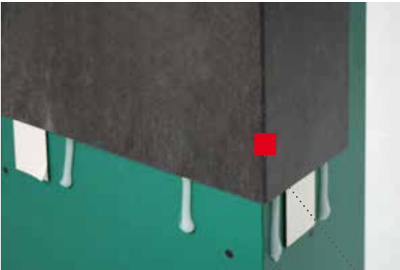
Outer edge created after milling the V-shaped groove on the back of the board
